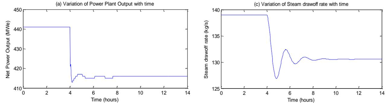
**Dynamic case study:** The response of the integrated plant with a step reduction in target power output.
