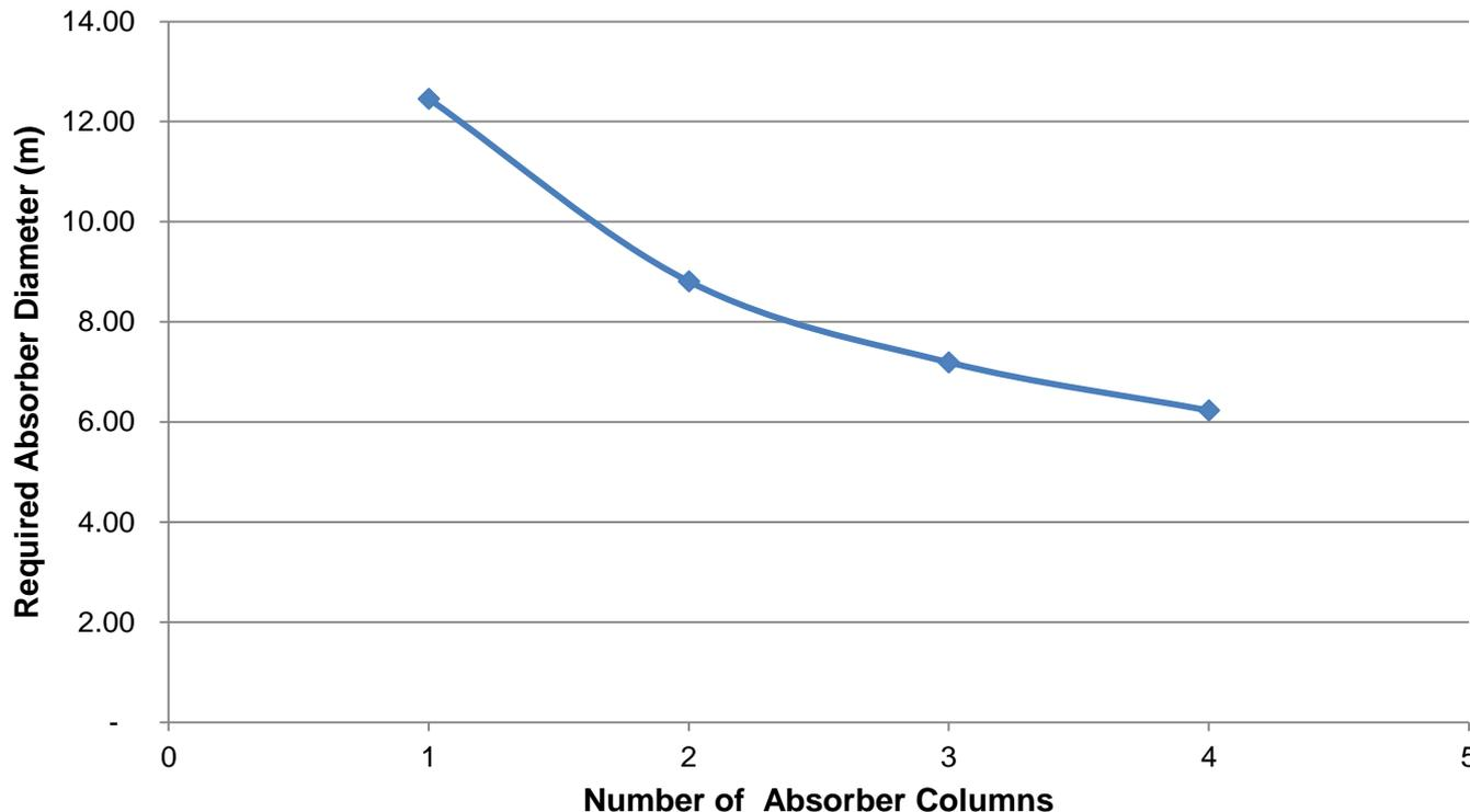
Column diameters should be below 12.2m (40feet)<sup>[2]</sup>
