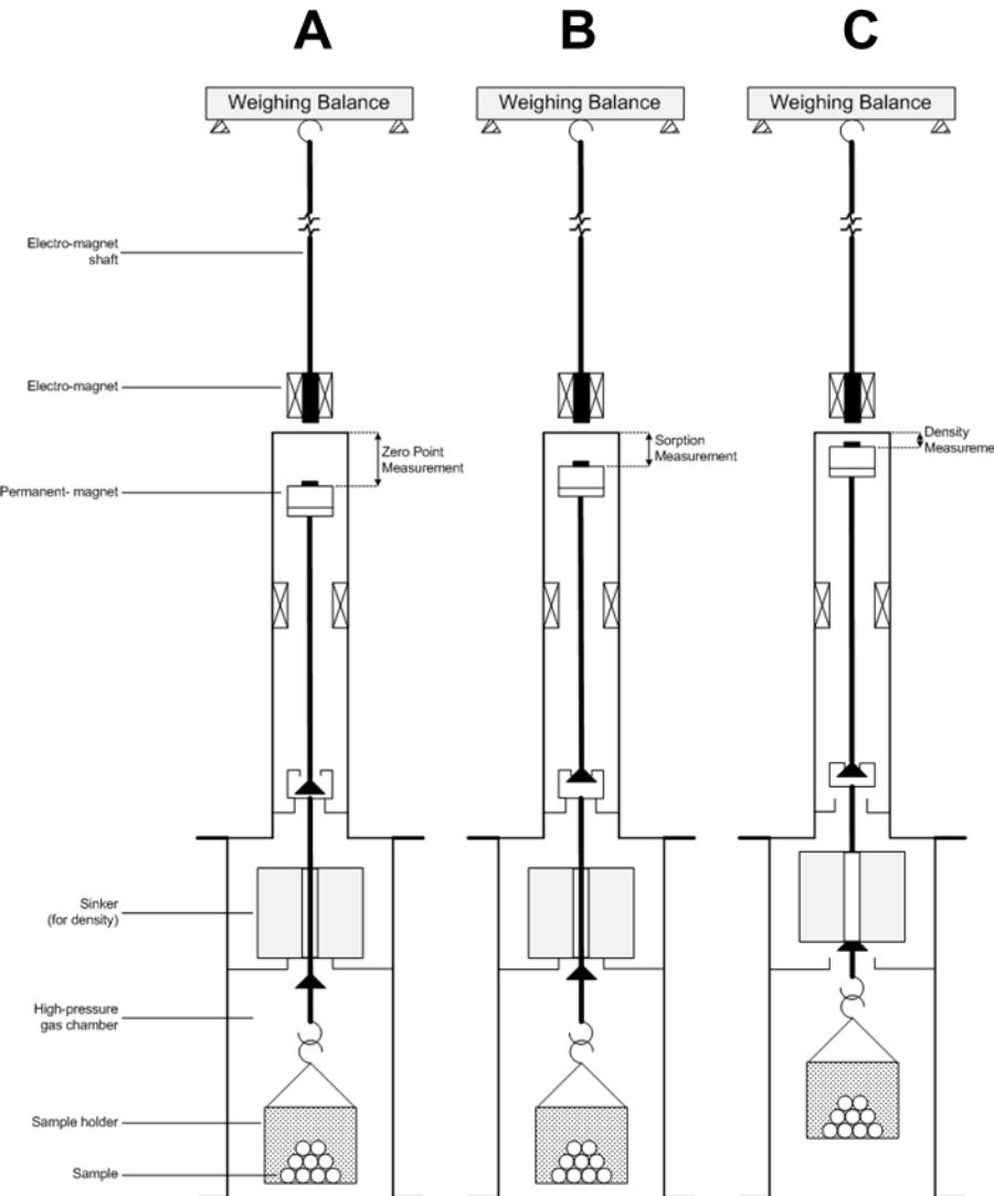
Schematics of magnetic suspension sorption apparatus operating principle. **(A)** sample loaded to measuring basket in high pressure cell; **(B)** Measurement point 1 (MP1) – magnetic coupling is on and mass of the sample is measured; **(C)** Measurement point 2 (MP2) – in-situ density of the adsorbed gas is measured.
