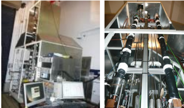
HIPOR rig - Crude oil fouling measurement in industrial conditions
