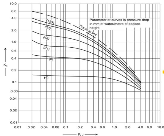
FIGURE 4.11: Generalized pressure drop correlation from Sinnott
