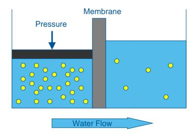
Pressure is applied to concentrated solution to overcome osmotic pressure and force water through the membrane from the high concentration side to the low concentration side
