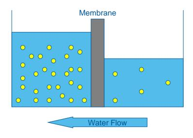
Water diffuses naturally through membrane from low concentration side to high concentration side
